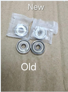
BLOWER BEARING RENEWAL
